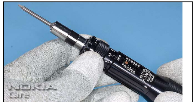
6. Use a torque driver for tightening the screws. Set the correct torque.
